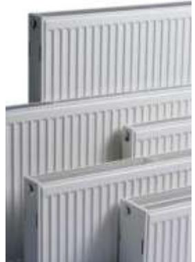
These panels are made of corrosion-proof low-carbon steel. Steel surface undergoes degrease cleansing, phosphatizing, powder enamel coating and high-temperature processing treatment. Panels have various height and width. So, one can make a unit of any heating capacity. Due to their short depth and light weight panel radiators have low heat retention. The great heating surface area of panels ensures the intensive movement of heated air. So, their share of convection heat transfer amounts to 75%.
